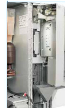
Protected compartment for payment systems. Coin mech or validator can be fitted together with a cashless system.
