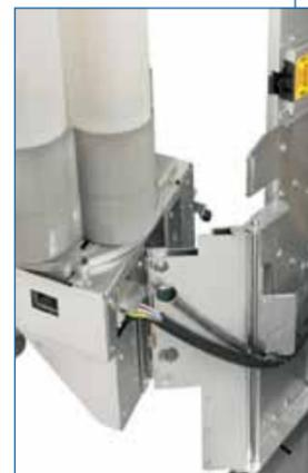
Easy internal access, even when banked, due to the 180° opening of the cup turret with double hinge
